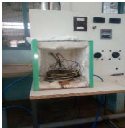
Fig.2.2. Guarded hot plate method experimental set up
