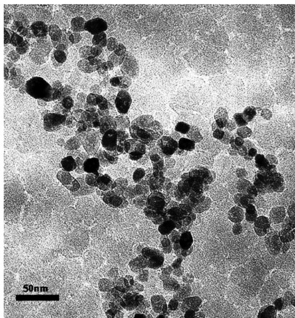
**Fig 3:** Transmission Electron Microscopy image of TiO<sub>2</sub> nanoparticles
