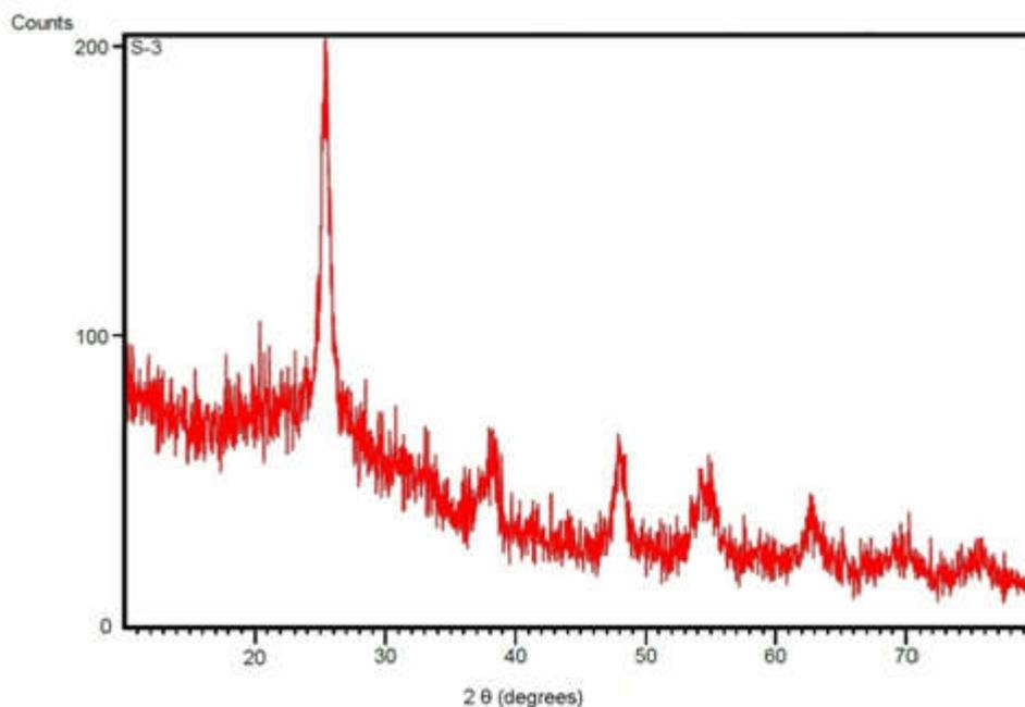
**Fig 1:** X-Ray Diffraction patterns of synthesized Titanium dioxide nanoparticles
