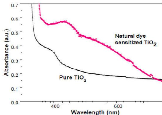
**Fig. 2 Absorption spectra of pure and natural dye sensitized TiO<sub>2</sub>**
