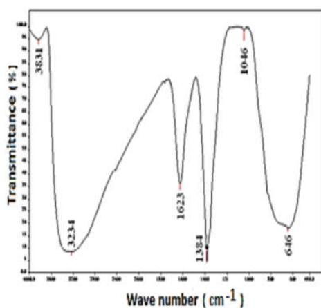
**Fig. 3a - FTIR spectrum of pure TiO<sub>2</sub>**
