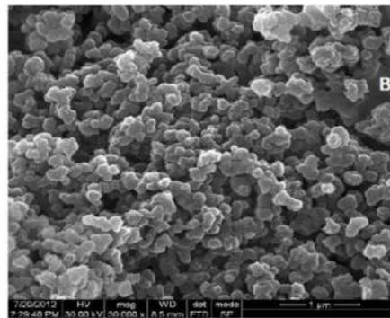
**Fig. 4b - SEM image of natural dye sensitized TiO<sub>2</sub>**
