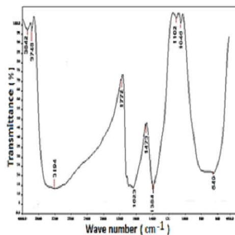
**Fig. 3b - FTIR spectrum of natural dye sensitized TiO<sub>2</sub>**
