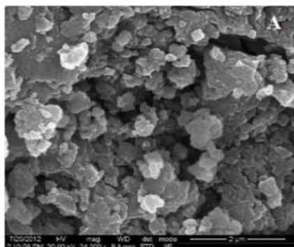
**Fig. 4a - SEM image of pure TiO<sub>2</sub>**
